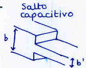
$$\frac{B}{Y_0} = \frac{2b}{\lambda_g} \left[ \ln \left( \frac{1-\alpha^2}{4\alpha} \right) \left( \frac{1+\alpha}{1-\alpha} \right)^{\frac{1}{2}} \left( \frac{a+t}{a} \right) + 2 \frac{A+A'+2C}{AA'-C^2} \right]$$
